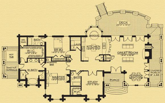
Special Notes: Without carport an walkout - 9' plus or minus first floor wall height, extra courses per plans, exterior log siding or half log for turret, full log corners in dining room front wall in lieu of stone columns, round truss and purlin roof system for porch, deck is not upgraded for hot tub, wood arch over entry included, ironwork is not included, front walls at offsets are less than 9' plus or minus.
