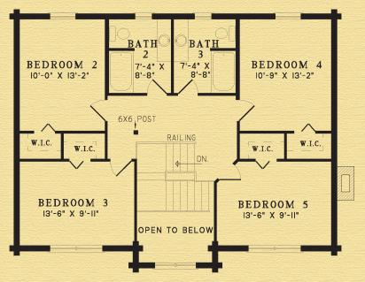
Special Notes: Has 8' plus or minus upper level wall height. One half circle window included. Garage walls and gable are frame with exterior log siding or half log with corners. With heavy timber rafter system and no roof insulation.
