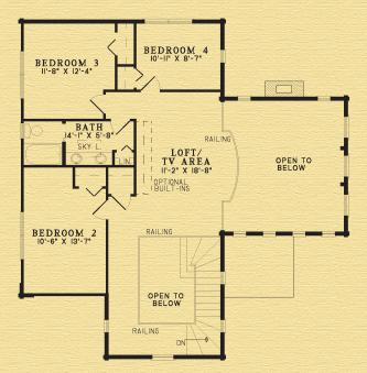
Special Note: 9' plus or minus & 10'-2" first floor wall height, 5'-6" second floor wall height. Two full circle windows included. Log Siding or half log for exterior of box bay.
