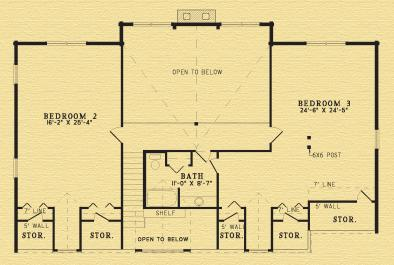
Special Notes: Has 7'-11" plus or minus log walls on rear of second floor. Full log gable and shed dormer. Log siding or falf log for one offset gable. One 3" arch included.
